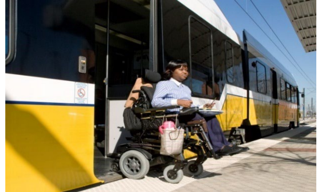
Level Boarding with Low-Floor Vehicle
